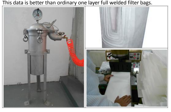
PGF bag is total 15 layers, covered with a layer of PP woven material, to make it easy for you to install the filter bag, as well as prevent fiber migration.
