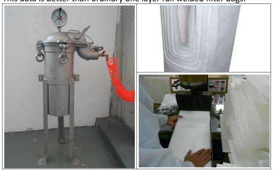
PGF bag is total 15 layers, covered with a layer of PP woven material, to make it easy for you to install the filter bag, as well as prevent fiber migration.
